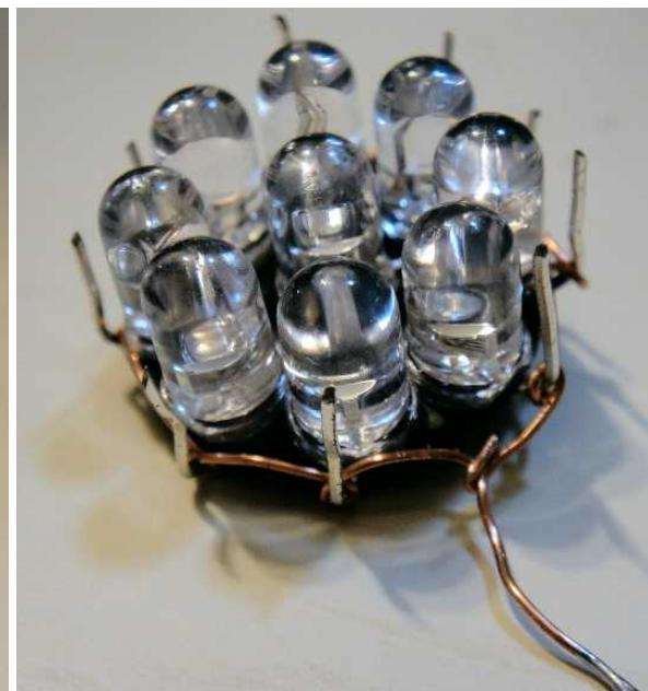
Fig. 16 – Negative leads need to be wired & cut.
