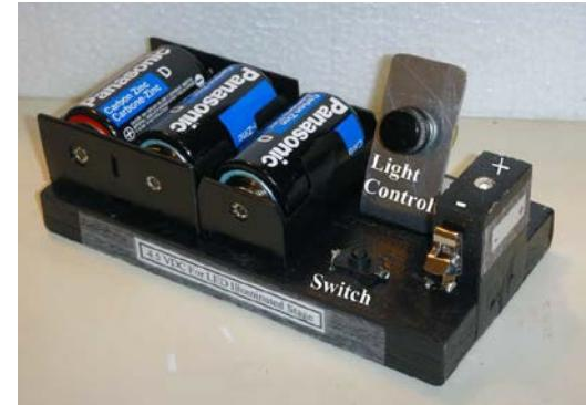
Fig. 21 – Stage variable power supply.
