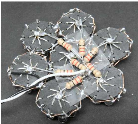
*F 17 – Current limiting 22 ohm resistors.*
