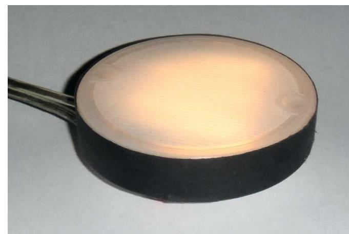
*Fig. 6 – Black paper reduces extraneous light. Note the color differences. It is really more of a warm white.*
