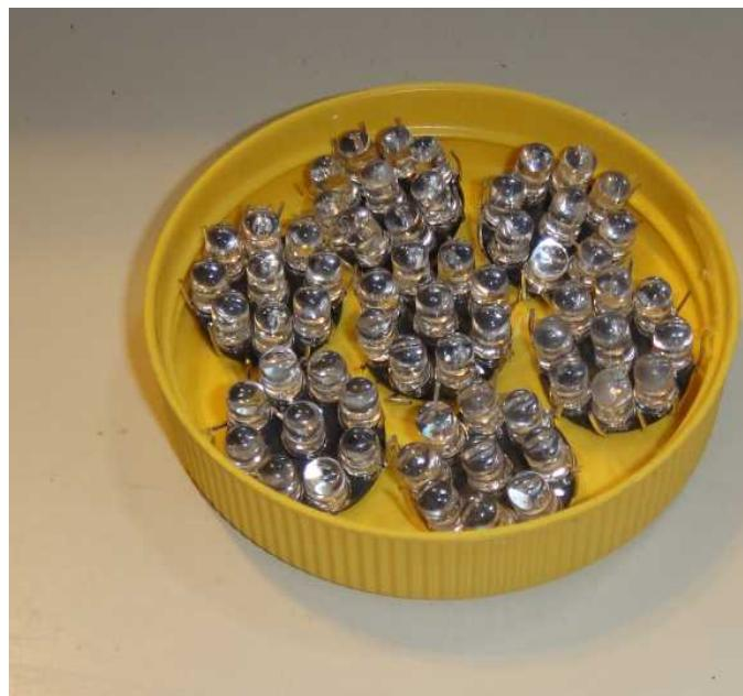
Fig. 15 – 7 LED assemblies fit in a plastic mustard cap.
