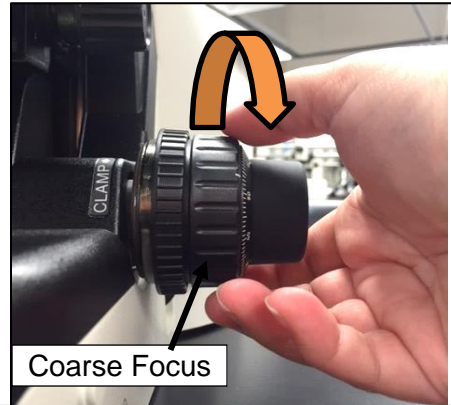
Figure 04. Lower the stage by turning focus knob counter-clockwise or your thumb at the 12 o'clock position and moves toward you.
