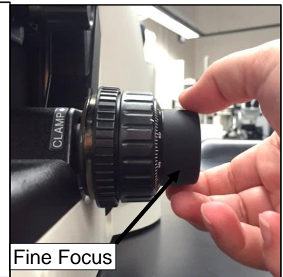
Figure 04. Lower the stage by turning focus knob counter-clockwise or your thumb at the 12 o'clock position and moves toward you.
