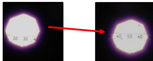
Figure 12. The polygon shape of the aperture is made by the leaves of the diaphragm. Each flat edge indicates one leaf.
