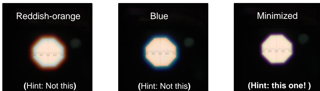
Figure 13. Under, over, and proper focus of condenser. Very important that you are still focused on the specimen plane at this point.
