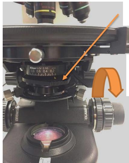
Move substage condenser diaphragm to fully close down.
