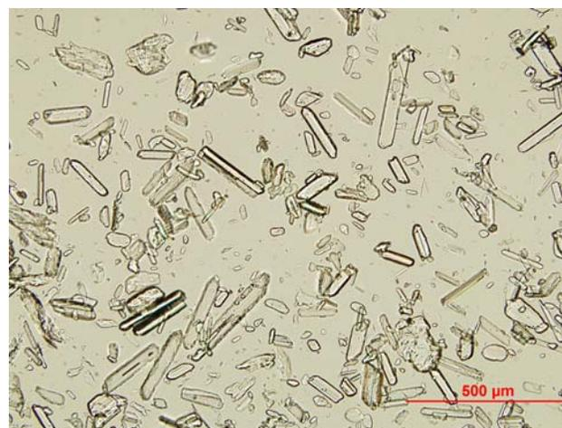
Figure 3-1. Salicylic Acid, plane-polarized light, 100X
