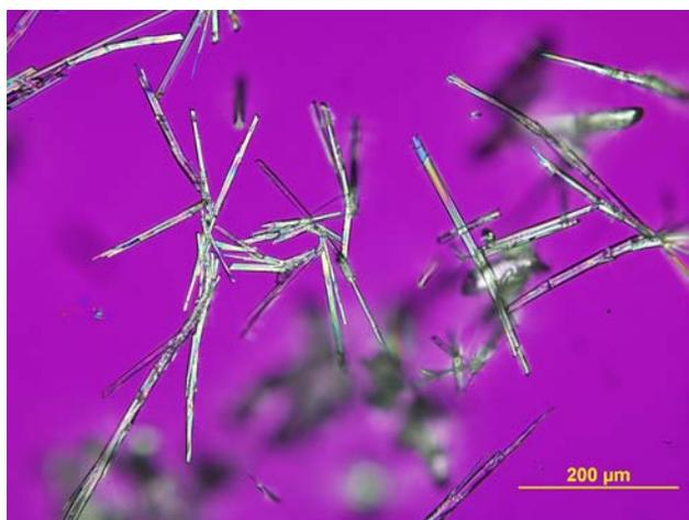
Figure 2-11. Salicylic Acid sublimite, crossed polarizers, first-order red compensator, 200X
