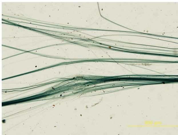
Figure 4-1. Fibrous Riebeckite, plane-polarized light, polarizer East/West - fiber length East/West, 100X
