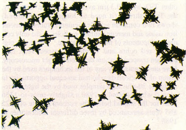
Figure 11 Microchemical test for Zn showing drusy crosses with potassium mercuric thiocyanate, 160x.
