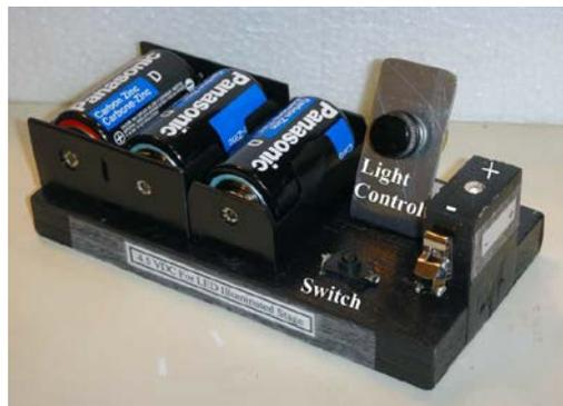
Fig. 21 – Stage variable power supply.
