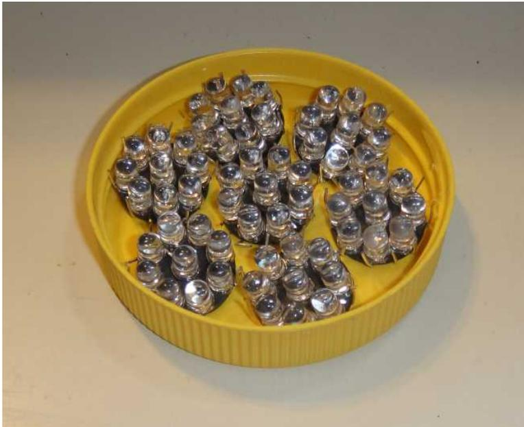
Fig. 15 – 7 LED assemblies fit in a plastic mustard cap.
