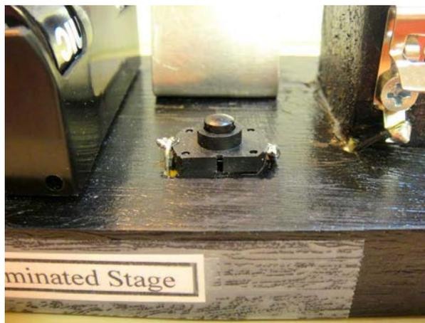
Fig. 22 – Flashlight Power Switch is used.
