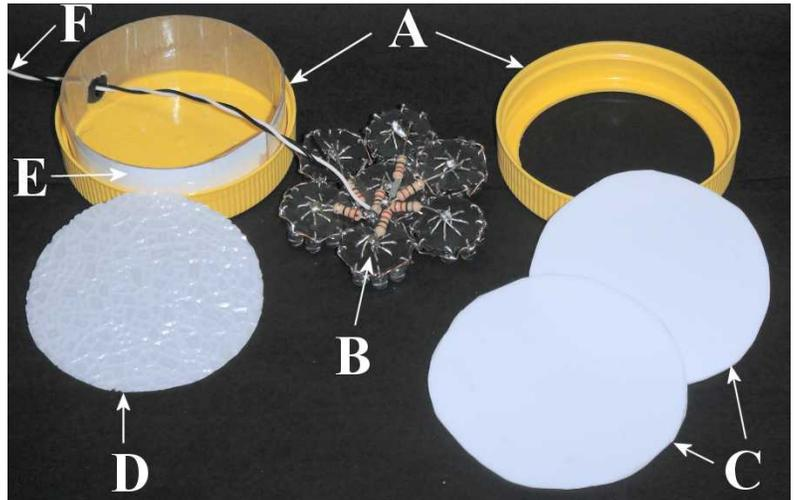
Fig. 18 – Parts for the LED illuminated stage.
