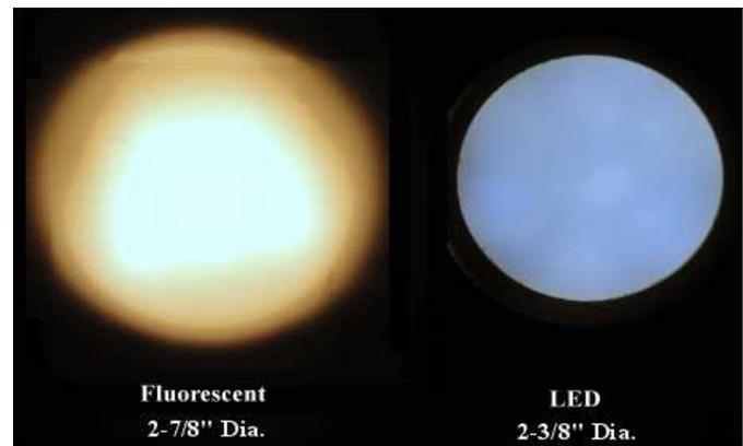
Fig. 19 – Two illuminated stages compared.
