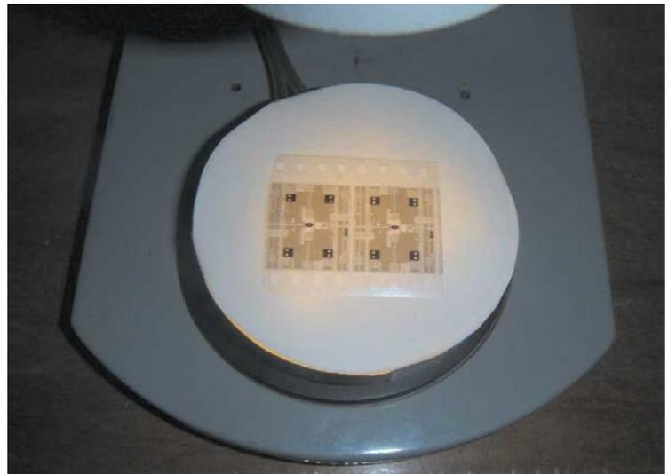
Fig. 9 – 35 mm film is back lit for a sharper image.
