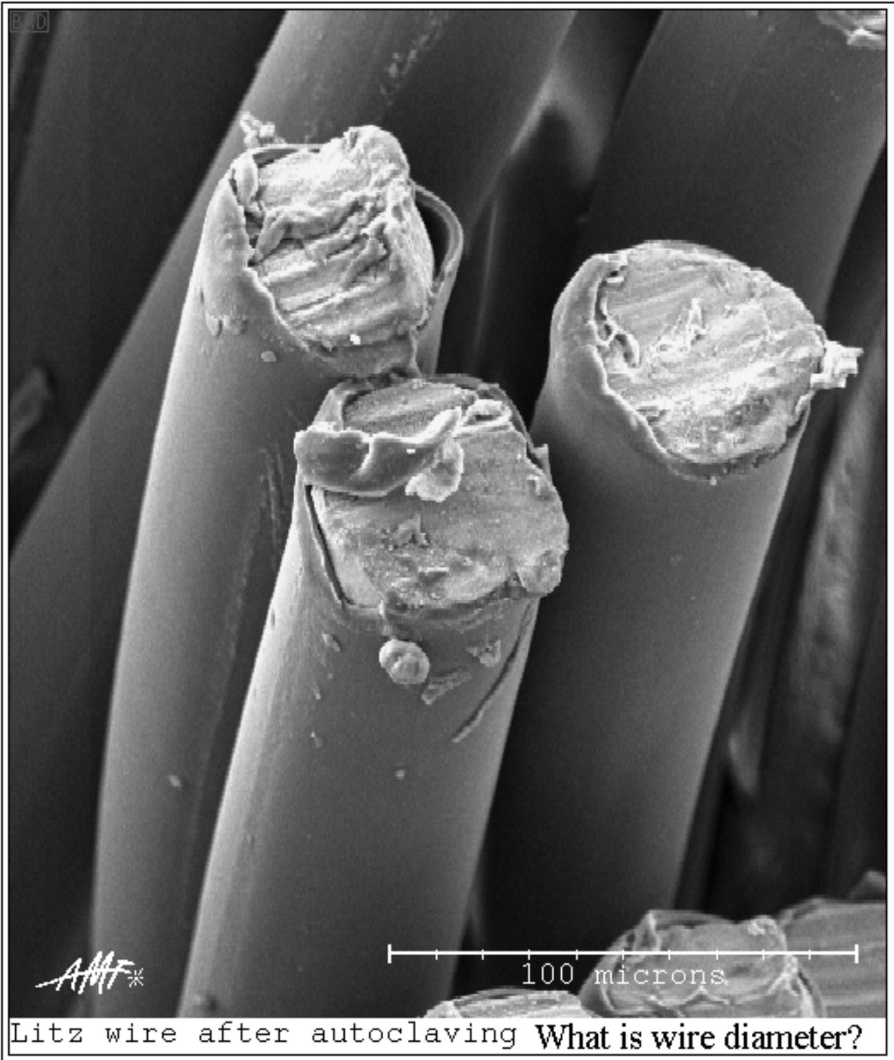
Figure 18 – Further magnification of the litz wire bundle shown in figure 17 within the area shown in the box.
