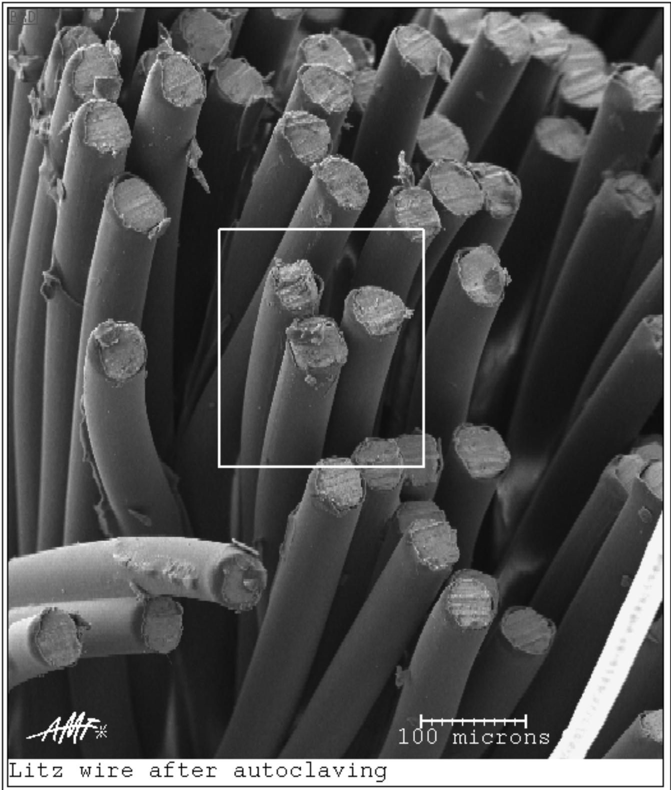
Figure 17 - Further magnification of the bundle shown in figure 16 within the area shown in the box.
