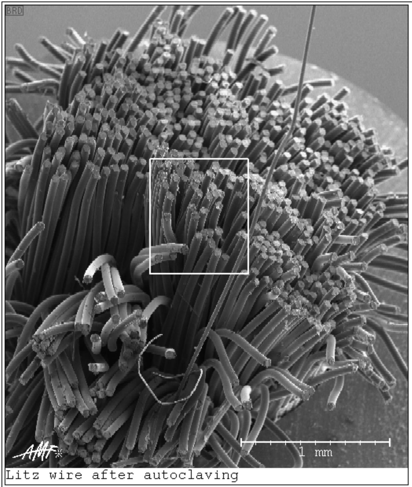
Figure 16 – SEM view of part of the end of a bundle of 44 Ga. copper wires used to wind a coil.
