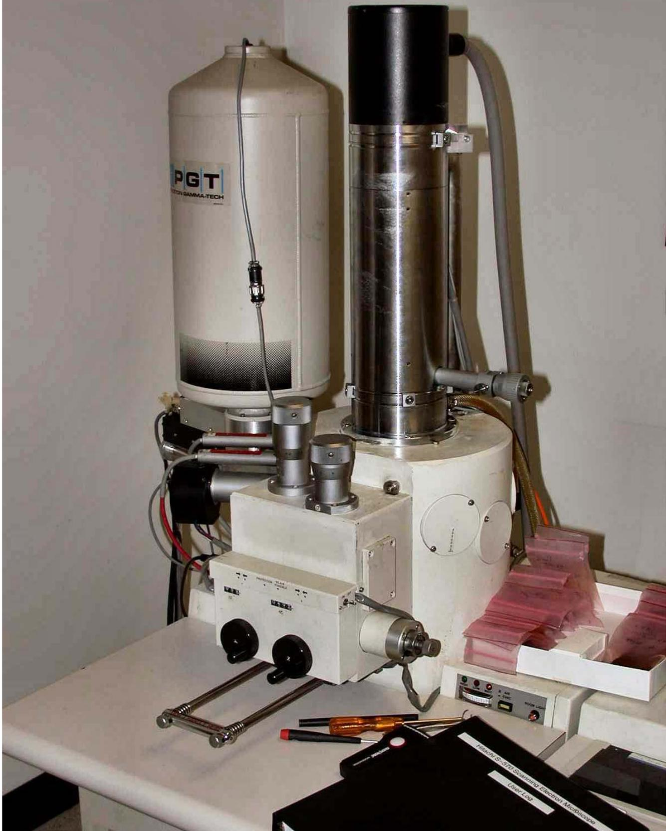
*Fig. 15 – Older style SEM that is quite “labor intensive” compared to more modern “production” instruments.*
