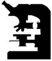
4. **While still looking from the side**, rack the stage to its highest point but **DO NOT ALLOW THE OBJECTIVE AND COVERSLIP TO TOUCH!** Once at the top look through the oculars.
