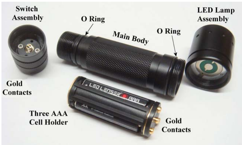
Fig. 5 – Waterproof Lenser D47852 flashlight assembly parts.
