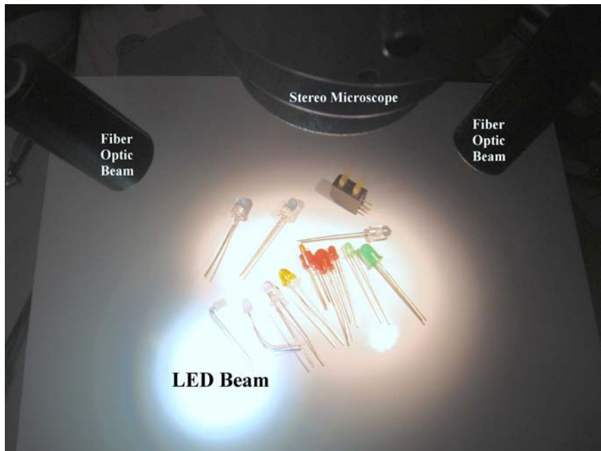
Fig. 1 – Normal 150 Watt halogen lamp light into two fiber optic cables.
